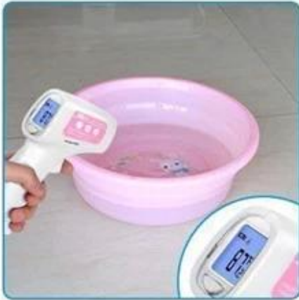
°F125.6(87°C) Hot water test
