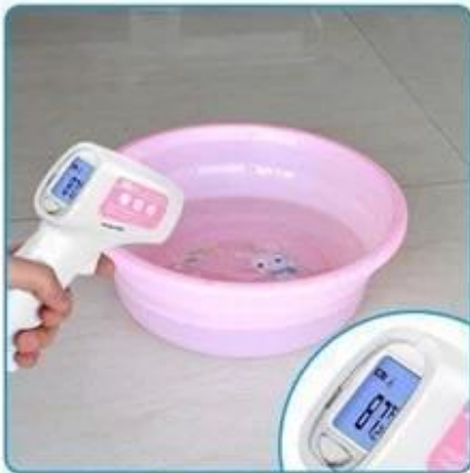
°F125.6(87°C) Hot water test
